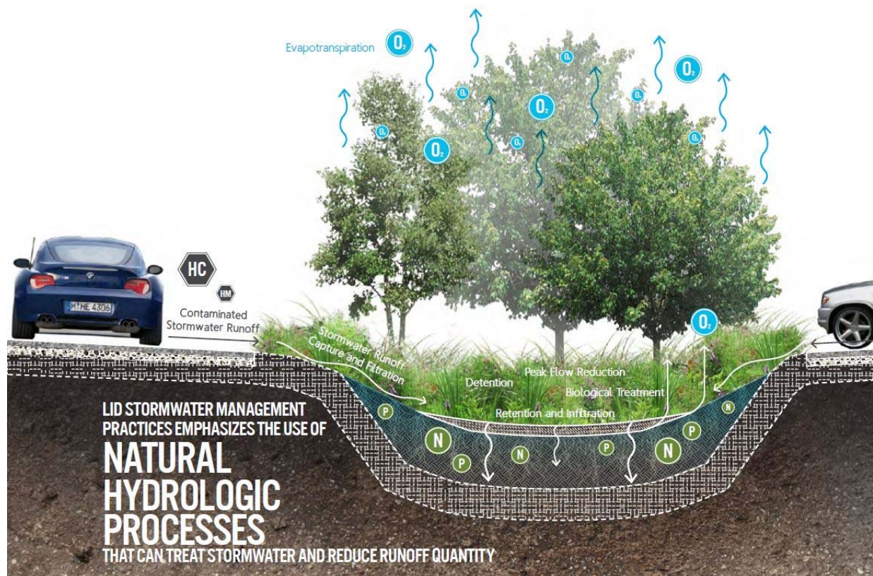
Slika 17: Shema upravljanja s padavinsko vodo z uporabo naravnih hidroloških procesov (Vir: B. Collett, V. Friedmann, W. Miller: Low impact development opportunities for the planet region, Knoxville-Knox County Metropolitan Planning Commission, 2013 )
